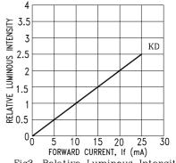
Fig3. Relative Luminous Intensity vs. DC Forward Current
